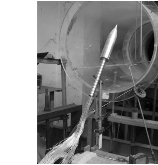
Fig. 2 Photographs of a) cone-cylinder model and b) wind-tunnel experimental setup.
